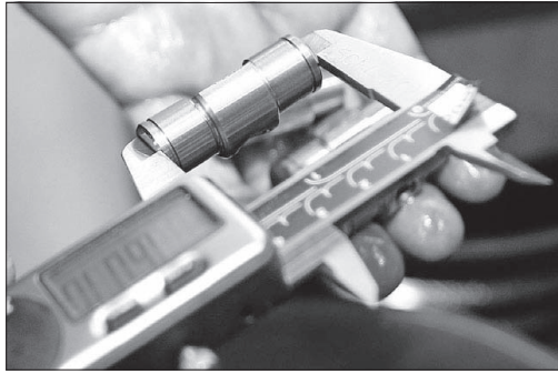
One highlight of the January employment report notes that the Ocala metropolitan statistical area posted the second fastest annual job growth rate compared to all other Florida metro areas in manufacturing, at 7.7 percent. In this file image from 2016, a worker at Scorpion Racing Products uses a dial caliper to check the dimensions of a trunnion for an aluminum roller rocker after it was manufactured at the Ocala facility. [BRUCE ACKERMAN/STAFF PHOTOGRAPHER/FILE]
